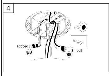
4. Strip 3/8" of insulation from the electrical wire ends. Using wire nuts (BB), connect RIBBED fixture wire to the WHITE supply wire from the outlet box; connect the SMOOTH fixture wire to the BLACK supply wire.
