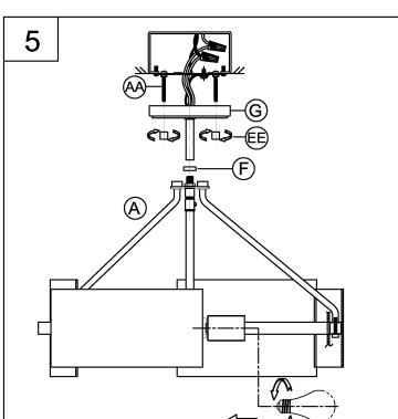
5. Attach seat ring (F) onto fixture (A), thread fixture (A) onto canopy to secure tightly.
