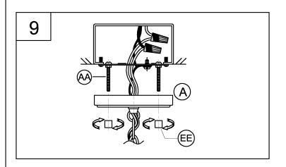
9. Secure the fixture (A) to screws (AA) use the two cylinder nuts (EE) to secure tightly.
