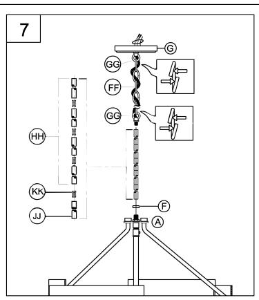
7. Pass the wires through the seat ring (F) / nipple (KK)/one pipe (JJ)/four pipe (HH) to achieve overall desired length.
