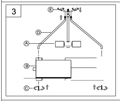
3. Attach round arm (D) to frame (B) use screw (C) to secure tightly; then attach other end of round arm (D) to the steel plate of fixture (A) use finial (E) to secure tightly.
