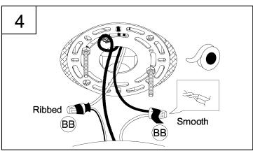
4. Strip 3/8" of insulation from the electrical wire ends. Using wire nuts (BB), connect RIBBED fixture wire to the WHITE supply wire from the outlet box; connect the SMOOTH fixture wire to the BLACK supply wire. Connect the fixture ground wire and supply ground wire using a wire nut or by fastening to the ground screw on the round mounting plate. Push all wire connections into the outlet box.
