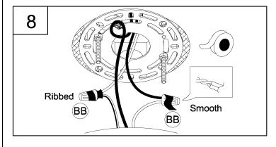
8. Strip 3/8" of insulation from the electrical wire ends. Using wire nuts (BB), connect RIBBED fixture wire to the WHITE supply wire from the outlet box; connect the SMOOTH fixture wire to the BLACK supply wire.
