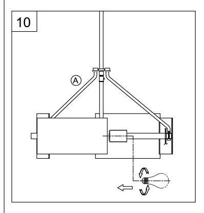
10. Screw lamp (not included) into fixture socket. Use 60-watt MAX incandescent medium base lamp, SBCFL or SBLED.
