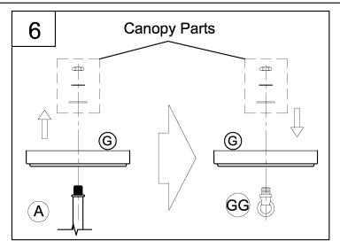
6. Remove existing canopy parts and canopy (G) from fixture(A).
