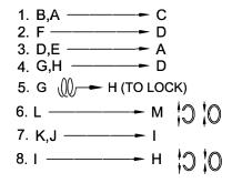
9. Thread Fixture Wires Up Through Chain, (K), (J). (H), (D). Trim Wires To Extend 6-Inches (15.5cm) Above (A). Strip Wire Insulation 1/2-Inch (1.5cm). Connect Fixture Wires To Supply Wires As Shown On Wiring Diagram.
