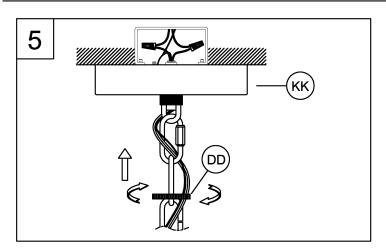
5. Tuck the wires into the junction box and slip the canopy (KK) over the chain holder. Thread the screw collar (DD) onto the chain holder to secure the canopy tightly to the ceiling.
