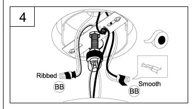
4. Strip 3/8" of insulation from the electrical wire ends. Using wire nuts (BB), connect the RIBBED fixture wire to the WHITE supply wire from the outlet box; connect the SMOOTH fixture wire to the BLACK supply wire.
