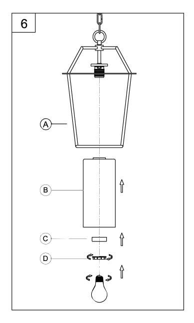
6. Attach the glass shade (B) and the socket cover (C) to the fixture (A) using the socket ring (D) to secure tightly.
