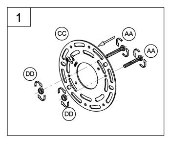
1. Loosely thread the screws (AA) and the hex nuts (DD) onto the swivel mounting strap (CC). You now need to adjust the screw length according to the fixture canopy depth.
