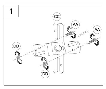
1. Screw screw (AA) onto swivel mounting strap (CC) and use hex nut (DD) to secure it tight.
