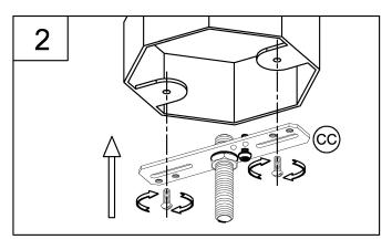
2. Attach assembled parts from Step 1 onto junction box, using the mounting screws supplied with the junction box (not included).
