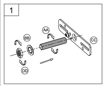
1. Screw nipple (AA) and lock washer(BB), hex nut (DD) onto mounting plate (CC).
