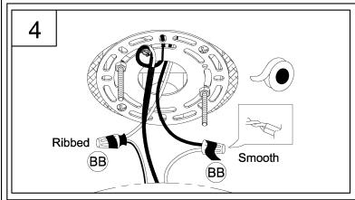
4. Strip 3/8" of insulation from the electrical wire ends. Using wire nuts (BB), connect RIBBED fixture wire to the WHITE supply wire from the outlet box; connect the SMOOTH fixture wire to the BLACK supply wire.
