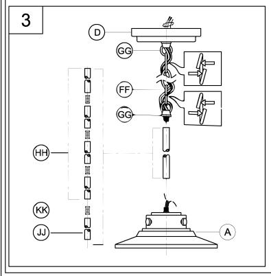
3. Pass the wires through the one pipe (JJ)/nipple (KK)/four pipes (HH) and chain loop (GG) to achieve overall desired length. Next attach pipes onto fixture (A) to secure tightly. Weave electric cord and ground wire through chain (FF) and canopy (D). Open two links of chain and attach both ends to chain loops (GG). Close the chain links.
