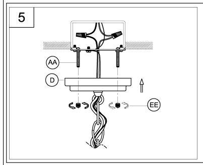
5. Secure the canopy (F) to screws (AA) use the two knurled ball nut (EE) to secure tightly.
