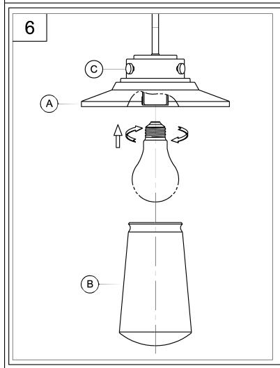
6. Screw lamp (not included) into the fixture socket. Use 60-watt MAX medium base lamp, SBCFL or SBLED.
