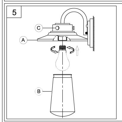
5. Screw lamp (not included) into fixture socket. Use 60-watt MAX incandescent medium base lamp, SBCFL or SBLED.
