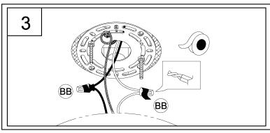
3. Strip 3/8" of insulation from the electrical wire ends. Using wire nuts (BB), connect white fixture wire to the white supply wire from the outlet box; connect the black fixture wire to the black supply wire.
