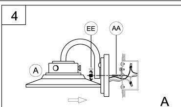
4. Attach fixture (A) to screws (AA) using knurled ball nut (EE). Secure tightly.
