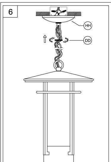
6. Tuck the wires into the junction box and slip the canopy(HH) over the chain holder. Thread the screw collar (DD) onto the chain holder to secure the canopy tightly to the ceiling.
