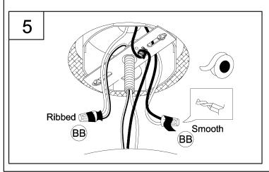
5. Strip 3/8" of insulation from the electrical wire ends. Using wire nuts (BB), connect RIBBED fixture wire to the WHITE supply wire from the outlet box; connect the SMOOTH fixture wire to the BLACK supply wire.
