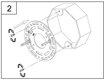
1. Screw screw (AA) onto round mounting plate (CC) and use hex nut (DD) to secure it tight.
