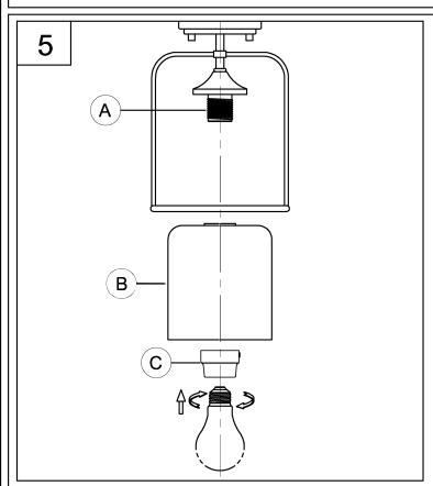
5. Attach glass shade (B) to fixture (A) and use socket ring (C) to secure tightly.
