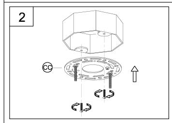
2. Attach assembled parts from step 1 onto outlet box using the mounting screws supplied with the outlet box (not included).
