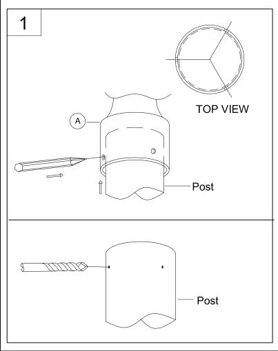
1. Place fixture (A) on post (not included) and use a pencil to mark the locations of the 3 mounting holes. Remove the fixture from the post and use a drill with a 0.144 (4mm) bit to create mounting holes in the post.
