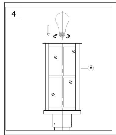
4. Screw lamp (not included) into fixture socket. Use 100-watt MAX incandescent medium base lamp, SBCFL or SBLED.
