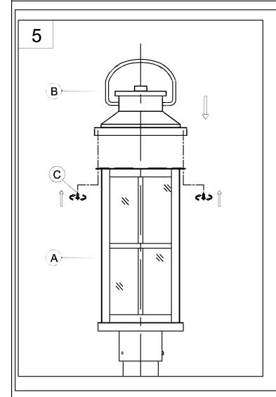
5. Attach the roof (B) onto the Fixture (A), use the screw (C) to secure tightly.
