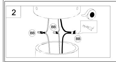
2. Strip 3/8 " of insulation from the electrical wire ends. Using wire nuts (BB), connect white fixture wire to the white supply wire from the outlet box; connect the black fixture wire to the black supply wire from the outlet box.
