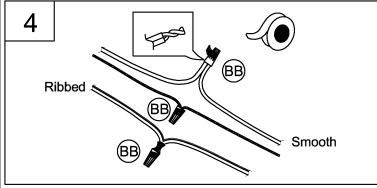
4. Strip 3/8" of insulation from the electrical wire ends. Using wire nuts (BB), connect RIBBED fixture wire to the WHITE supply wire from the junction box; connect the SMOOTH fixture wire to the BLACK supply wire.
