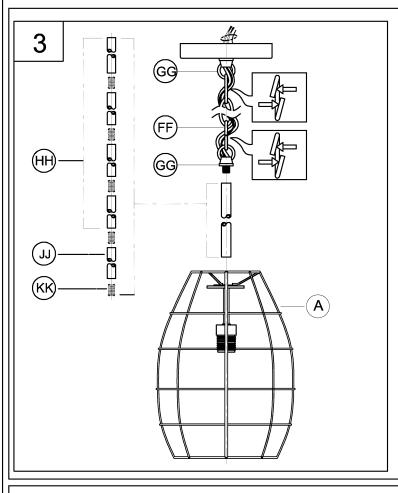
3. Pass the wires through the nipple (KK)/one pipe (JJ)/four pipe (HH) and Chain loop (GG) to achieve overall desired length. Next attach pipe onto fixture (A) use nipple (KK) to secure tightly.
