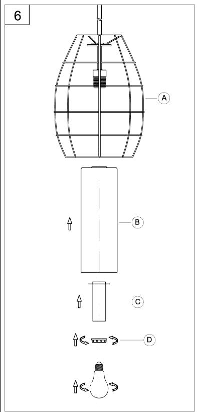
6. Attach glass shade (B) to fixture (A) using socket spacer (C) and socket ring (D) to secure tightly.
