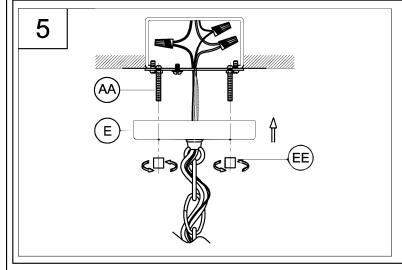
5. Secure the canopy (E) to screws (AA) use the two cylinder nuts (EE) to secure tightly.
