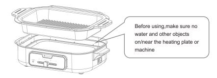
4. Connect the power plug into the machine. Plug the power cord into the wall socket and you are ready to use your electric grill. (Note: Make sure the voltage which is indicated on the machine matches the local voltage before connecting the machine.)
