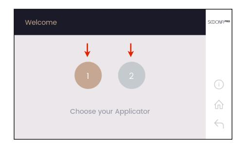
Choose applicator 1 or 2, if both applicators are plugged in, select one to set up first and then set up the second applicator (see page 8)
