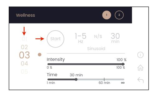
On the left side of the screen scroll through the numbers to the desired program and push the START button, the program will start after a few seconds
