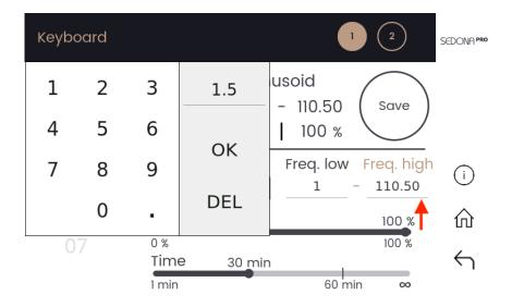
Type in the desired amount in the keypad for the low frequency and press OK to set. Do the same for high frequency if desired
