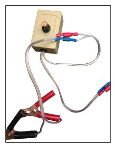
Attach the manual control to the leads to the motor and to the battery clips provided. The connectors are color coded DO NOT hook them up backwards.
