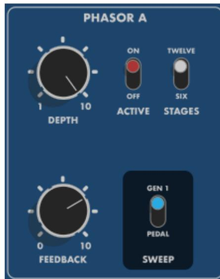
The **ACTIVE** switch reproduces one of the two footswitches present on the original hardware. If the switch is off, the phasor is bypassed and has no effect on the signal. Sometimes it is useful to turn on only one phase shifter at a time, either to create a subtler effect or to more clearly hear exactly what you're doing as you turn the knobs and flip the switches.
