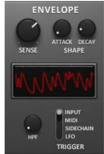
In the MIDI mode, the **SENSE** knob acts as a threshold control. If the velocity of a note is below the setting of the **SENSE** knob, the note is ignored. If you leave the **SENSE** knob at its full anti-clockwise setting, all notes generate gate signals for the envelope generator. Turning the **SENSE** knob up raises the threshold, blocking notes with low velocities and passing notes with high velocities.
