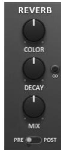
The switch labeled **PRE** and **POST** changes the signal path within Mangleverb. If the switch is set to **PRE**, the reverb comes before the filter and VCA. If the switch is set to **POST**, the signal passes through the filter and VCA before entering the reverb.
