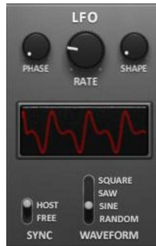
randomly determined shapes. The **SHAPE** knob changes the basic waveform in different ways, depending on which waveform is chosen with the switch.
