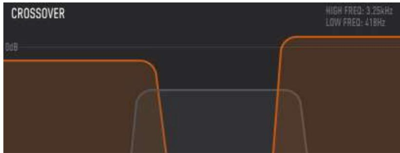
The height of each region controls the level (loudness) of the frequency bands. Click and drag vertically near the top edge of a band to increase and decrease its gain. There is also a handy Gain knob for each band at the bottom of Kombinat's window. The horizontal grey line near the top of the control represents 0dB, or unity gain.
