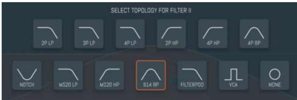
The icon labels use the conventions of "P" for Poles and "LP", "HP", and "BP" for Low-Pass, High-Pass, and Band-Pass. For example, the icon labeled 4P BP selects a four-pole band-pass filter. Here are descriptions of each of the filter types:
