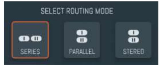
Filterstation uses separate filters for the left and right channels, so a stereo signal path is present regardless of the routing configuration.
