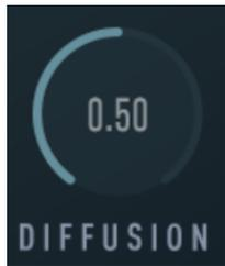
The **DIFFUSION** knob controls how much the initial density of echoes (often known as early reflections) builds up over time. Turning up the diffusion increases the build-up of echoes immediately following the original signal. High diffusion settings work well for percussion, but may sound too cluttered for vocals and full mixes.
