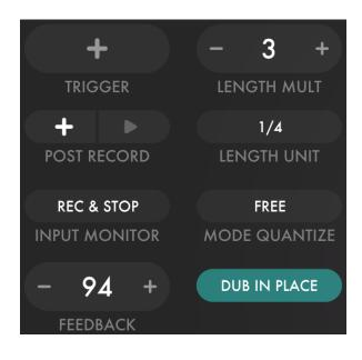
**TRIGGER** button (not the **RECORD** button). The length of the resulting loop will be equal to the setting of the **LENGTH UNIT** control multiplied by the value set with the **LENGTH MULT** control. To make a slightly contrived example: if **LENGTH UNIT** is 1/4, **LENGTH MULT** is 8, and **MODE QUANTIZE** is Measure, and you click the trigger, Enso starts recording when your host reaches the beginning of the next upcoming measure, records for exactly two measures, and then ceases recording.
