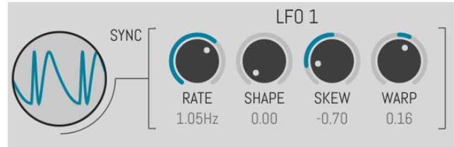
The **RATE** knob controls determine how fast the output of the LFO varies over time. They operate either in units of frequency (Hertz, or cycles per second), or in metrical units. The LFO's rate can be set from one cycle every 100 seconds (or 0.01 cycles per second, abbreviated 0.01 Hz) to 14 cycles every second (14 Hz). Click on the word **SYNC** to switch between the two modes.
