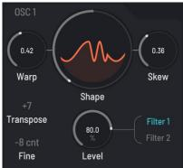
When the knob is rotated anti-clockwise, it acts as a sort of intensity control for the **Warp** and **Skew** knobs. This means that if the **Warp** and **Skew** are both set to zero, moving the **Shape** anti-clockwise won't change the oscillator's output; it will remain a sine wave. By contrast, the **Shape** knob itself changes the oscillator's tone when it is rotated clockwise from the center position.
