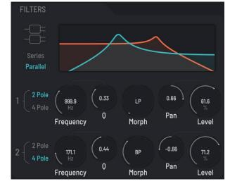
Finally, the buttons labeled Serial and Parallel change the filters between the serial routing and parallel routing. Filter Two follows Filter One when they are connected in series.
