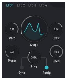
The Phase knob positions the FLFO's wave relative to either the start of the note, or to the host DAW's transport position. The setting of the Phase knob corresponds to the left end of the wiggly red line. If **Retrig** is turned on, the FLFO will start its cycle at this point on the wave when a note starts. If **Sync** is
