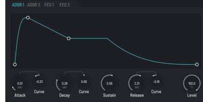
The FEGs can also be synchronized to the host DAW's tempo and transport; click the **Sync** button on the right to activate this synchronization. When sync is on, the segment durations are expressed in multiples of 1/32nd of a beat and can be as long as a full measure. Note that when sync is on, the time scale within Continua's window is linear.
