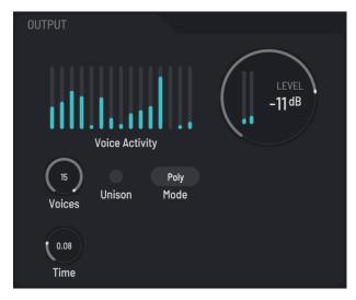
The **Voices** knob lets you set the number of voices, with a maximum of 15 (six when using the iOS version), that play simultaneously. Besides setting the number of voices that play in Unison mode, you can use this control to reduce the maximum CPU load of the plugin. This knob cannot be modulated.
