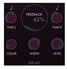
The TIME L and TIME R controls change the amount that signals are delayed in relation to the original (dry) signal. Each delay has a range of zero to two seconds.
