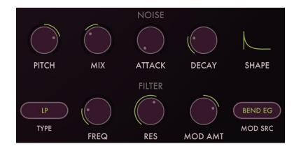
The MIX knob blends the metallic signal with the white-noise source. With a setting of 0%, you hear only the metallic sound; with a setting of 100%, you hear just the noise. In-between settings give you a blend of both.
