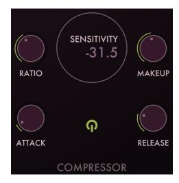
The **SENSITIVITY** control sets the level at which the compressor starts to engage or reduce the gain of the signal. Any signal level that exceeds the threshold will be compressed according to the ratio setting. The value displayed is in decibels relative to a full-scale signal, so *lower* values mean that the compressor is more likely to affect the signal. Drag vertically on the Sensitivity control to change the value.
