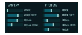
Drag the **ATTACK** and **RELEASE** sliders to the right to increase the attack and release times respectively. The **ATTACK CURVE** and **RELEASE CURVE** sliders vary the shape of the envelope from concave on the left to convex on the right, and linear in the center.
