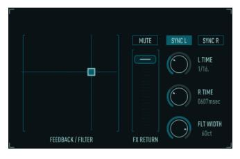
Dragging it to the left moves the filter frequencies downwards, making the delayed signal darker; dragging it to the right moves the frequencies upwards, making the delayed sound brighter.
