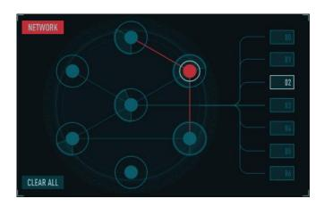
You can connect any neuron to any number of other neurons. The only restriction is that you cannot connect neurons such that the connections create a loop. Axon checks for loops as you make connections and will prevent you from forming loops.
