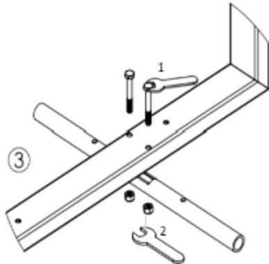
Hold Wrench in place while turning the 1st wrench
