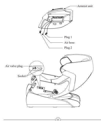
► Hold the armrest unit up and hook the bracket 2 onto the carrier groove, slowly push the armrest unit back into the chair linkage until bracket 2 aligns completely with bracket 4, insert bracket 1 into bracket 3, use a screw to secure the armrest into place. (Same installation method with the other side)
