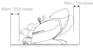
▶ Keep the distance between the power socket and power switch within 1.5 meters.
