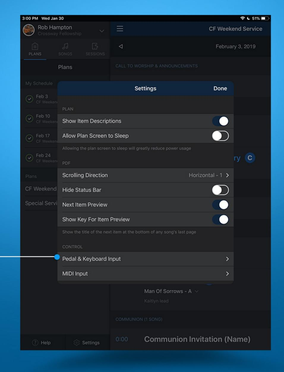
With your STOMP—Bluetooth Pedal powered on and paired with your tablet, select the command function you wish to adjust.
