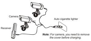
3. The camera can work during charging. Press the Power ON/OFF button to power on (turn on off) the camera, then you can use it.
