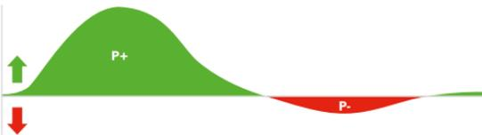
**PEDAL SMOOTHNESS (left leg):** used to interpret if the pedal stroke is rounder or more piston-like, its value being the ratio between the total torque and maximum torque of each cycle.
