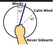
Throw no more than 45° from vertical. Each model may require a different angled thwor. A good rule is as wind increases, com up closer to vertical.
