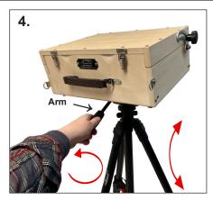
**4. Head Angle:** To adjust the angle of the Tripod Head to tilt your box forward or backward, twist to loosen the Arm and tilt it up or down to the angle you prefer before tightening the Arm again.
