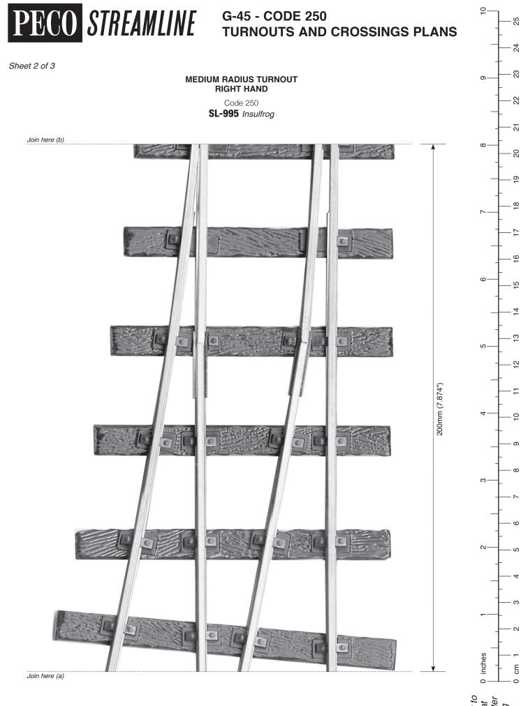
These plans are produced by the manufacturers and may be reproduced by modellers for the purpose of layout building. Commercial copying or reproduction prohibited. © PRITCHARD PATENT PRODUCT CO. LTD, BEER, DEVON EX12 3NA ENGLAND Use this scale bar to check that your printer is printing at 100%
