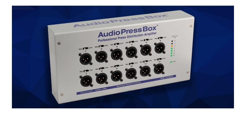
**APB-112 OW-D** is designed for use as a distribution audio amplifier for press conferences. It features one digital input from Dante network and twelve analog audio outputs with individual output level switch – MIC/LINE. There is no signal processing inside. All desired processing should be done in other devices (e.g. mixing console or DSP). So, the APB-112 OW-D is suitable for fixed installations with integrated Dante network.
