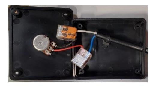
Disconnect the Wagos from the wires of the driver by lifting the orange arm to a 90-degree angle to release the wires.
