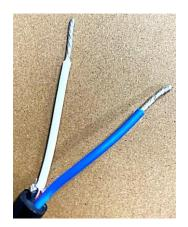
Meanwell drivers will have a blue (Dim+) and white (Dim-) wire.
