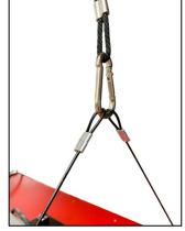
Gather both hanger cables and insert in the ratchet strap carabiner. Ensure the carabiner is closed completely
