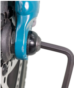
Loosen the front wheel axle bolts
