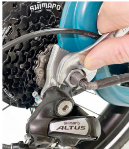
Loosen the rear wheel axle nuts
