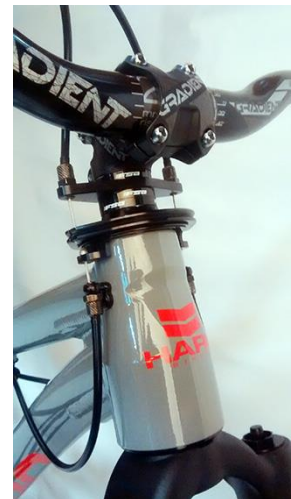
#2: Correct rotor plate position between 2 nd and 3 rd 5mm spacer
