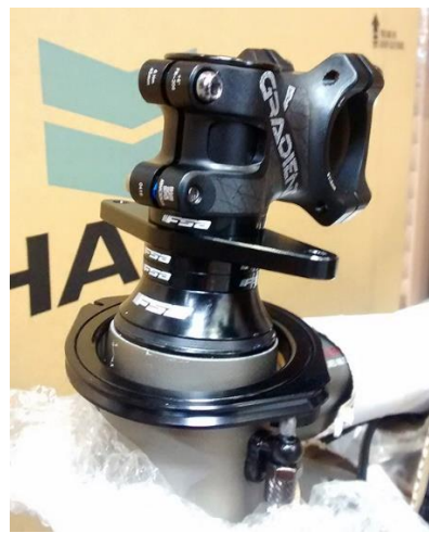
#2: Correct rotor plate position between 2 nd and 3 rd 5mm spacer
