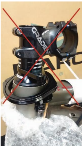
#1: Wrong rotor plate position Inside the box
