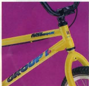
HEADTUBE GUSSET A Haro trademark. Wrap around reinforcement where it's needed most.
