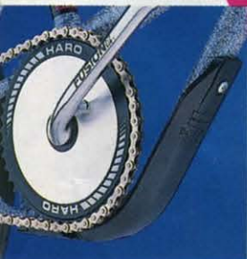
BASHGUARD The first of its kind. Lightweight replaceable alloy sprocket protection.
