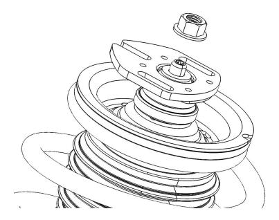
12. Assemble the camber/caster kit onto the strut as illustrated below. If you would like to lower the front by ½", remove ride height spacer from assembly and replace M8x35mm screws with supplied M8x25mm. If you would like to keep ride height unchanged, leave ride height spacer in assembly along with M8x35mm screws.
