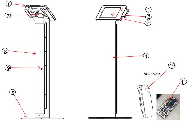
(1) iPAD Enclosure (2) iPad (3) Lock (4) Stand (5) Base (6) Micro usb port (7) Card Holder (8) Back Door (9) Lock (10) Credit card reader case (11) LED Remote Control
