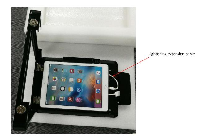
Step 5 Put the iPad into the enclosure, connect power cable to the iPad (if not using credit card reader), close the front cover and lock it.
