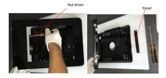
Step 5.2 Connect provided usb cable from power supply to the credit card reader, Install the Credit card reader inside the Case.
