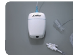
Sidestream CO 2 module sampling at <50 mm/sec. Perfect for your smallest patients or horses with large ET tubes
