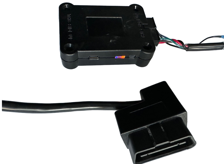
The image below displays both ends of the device cable: one end to the device and the other to the OBDII port.
