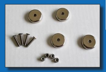
To attach the magnets to the device, insert one of the screws through a magnet and into one of the installation holes. Then, thread one of the nuts onto the screw and tighten. Repeat the process until all magnets and hardware have been used. Be careful not to over-tighten to avoid breaking or cracking the device casing.
