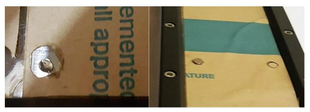
**PLEASE be patient with the drying of the adhesive!** If you do not put enough or rush the drying process of the adhesive to the magnet you will not have a strong bond and will soon see magnets sticking to the light bar or the lens cover.
